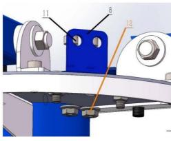
7.Hang the spring(23)on the screen clamp(5),hang the hooked end of the flower basket(22)on the spring hook plate(8),hook the looped end of the flower basket(22)with the spring(23),and then level the arm support
