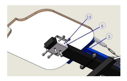
10.Lock the socket head cap screw(13) on the base disc(as shown in the figure), and stick the felt pad(21) onto the head end of the socket head cap screw(13). Use the tool wrench 14- 17(I)
