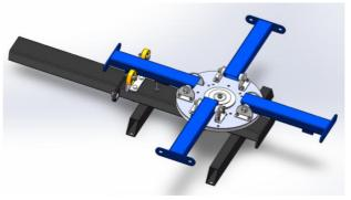
4. Take the screen clamp(5) and stick it to the printing arm(2), insert it into the printing arm(2)hole from the screen clamp(5) with square neck bolt M10X20 (16), and put the other end on the sleeve with gasket M10(17), then lock the outer hexagon nut M10(18), and then use wrench 14 - 17(I) to lock it
