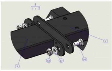
2. Put the positioning seat(4)on the square tube of the base(1),thread it from top to bottom with the external hexagon screw M8X55,and lock the other end with the external hexagon nut M8. Put the outer hexagon screw M10X55(15) onto the outer hexagon nut M10(18)and thread the screw head 40 mm from the base square tube from top to bottom, then lock the outer hexagon nut M10 (18)onto the base square tube in reverse.
