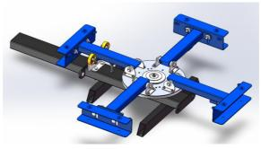
5.Lock the five-star handle(19)into the screen clamp (5)with a depth of 20mm,cover the pressure plate(20),and then use a cross screwdriver(2) to lock the pressure plate(20)on the five-star handle(19)with a cross countersunk screw M4X8(9)from the small hole at the lower end of the screen clamp(5)
