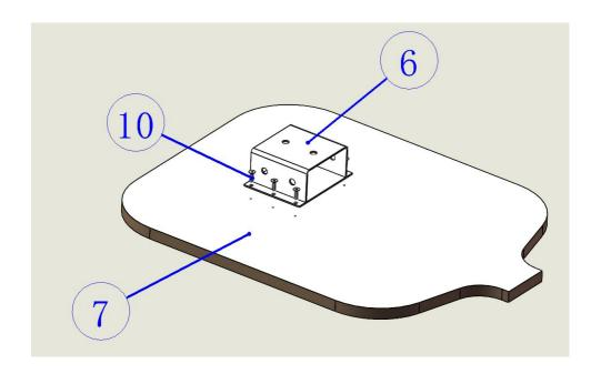
9.Insert the bracket(6)in the bracket of the wooden plate assembled in step 8 into the plate support bar(3),and then insert the socket head screw M10X30(14)into the tooth hole of the bracket(6),and then use the socket head wrench M10(five)to lock the socket head screwM10X25(14)
