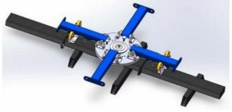
4.Take the screen clamp(5)and stick it to the printing arm(2), insert it into the printing arm(2)hole from the screen clamp(5) with carriage screw square M10X50(16),cover the other end with gasket M10 (17),then lock the outer hexagon nut M10(18),and then lock it with wrench 14-17(—)
