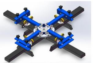
7. Put the spring hook plate(8) on the base disc, and lock it with the hexagonal socket screw M6X16 and flange nut M6
