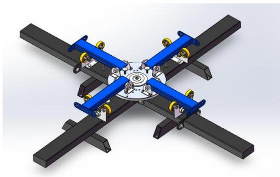
5. Take the screen clamp(5) and stick it to the printing arm(2), insert it into the printing arm(2) hole from the screen clamp(5) with square neck bolt M10X20(16), cover the other end with gasket M10 (17), then lock the outer hexagon nut M10(18), and then lock it with wrench 14- 17(一)
