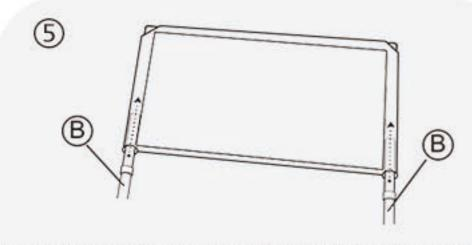
Insert the two columns into the screen and attach them to the joint.
