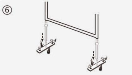
Insert the two posts into the base and lock them firmly.
