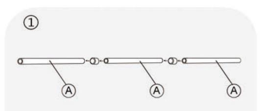
Connction 3 longaluminum tubes and assemble top bar with straight plastic parts.
