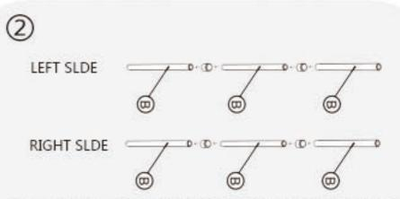
Assemble the left and right columns by connecting 3 short aluminum poles with straight plastic pieces.
