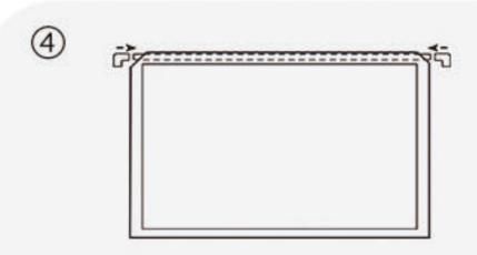
Insert and secure the connector at both ends of the bar and screen.
