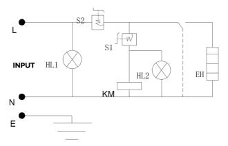
S1-Thermostat HL1-Power Light KM-AC Cont Actors S2-Temperature Limiter HL2-Heating Light EH-Heating Pipe
