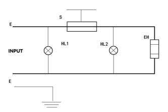
S-Temperature Controller E-Ground Protection HL1-Power Indicator(GREEN)
