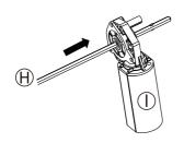
First, insert the motor from the end of the hexagonal rod without a bump to the other end with a bump.
