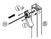
Then, insert the convex end of the motor into leg B together with the motor. Tighten the motor on leg B with the screws shown in the picture.
