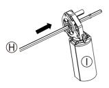
First, insert the motor from the end of the hexagonal rod without a bump to the other end with a bump.
