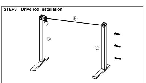
After completing the previous step, insert leg C into the hex stick.
