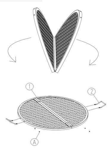
Spread out the grill in the arrow direction and lock the handle with M6 hex nut
