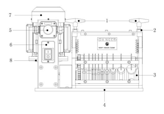
1:M12 Plastic screw 2:Nut for regulating blade up and down
