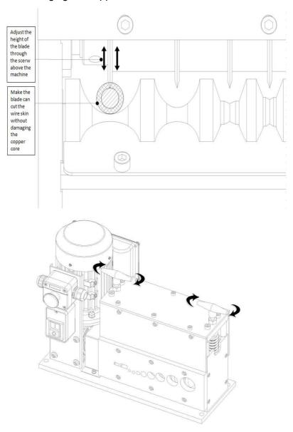
As the different thicknesses of the wires/cables, we need to adjust the blade up and down by adjusting the two M12 plastic screws on the machine (the blade goes down if you turn clockwise and the blade goes up if you turn counterclockwise)
