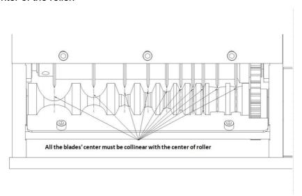
3.According to the thickness of the wire, adjust the height of the blade through the screw above the machine so that the blade can cut the wire skin without damaging the copper core.
