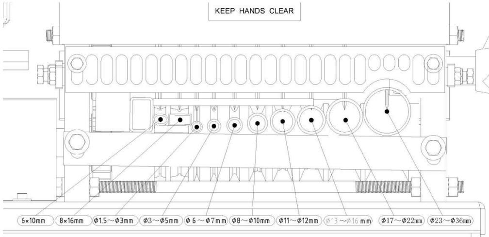
2. During wire stripping, the center of the blade must be collinear with the center of the roller.
