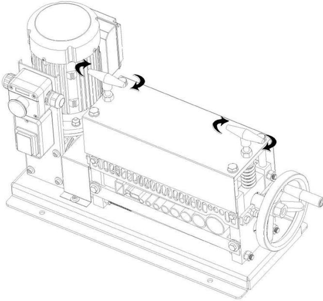
4.As the different thicknesses of the wires/cables, we need to adjust the blade up and down by adjusting the two M12 plastic screws on the machine (the blade goes down if you turn clockwise and the blade goes up if you turn counterclockwise)
