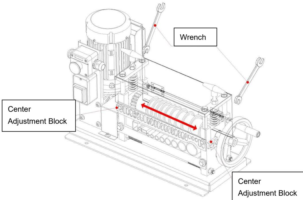
Adjusting the center adjustment block to adjust the blade shaft to the left or right by the wrench.
