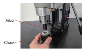
3. Loosen the chuck's jaws by inserting the chuck wrench (E) into either hole on the chuck and turning it counterclockwise.
