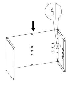
Step 2: Align bottom's(5) and hang bottom panel's(10) holes to left and right side panel' bottom holes, and secure them with (13)M6x15.
