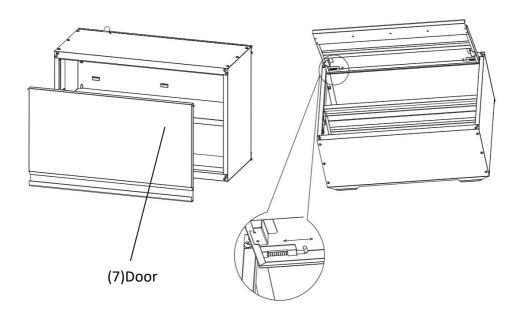
Before installing the gas spring (11), it is necessary to disassemble the spring support (as shown in the figure), install the base and the pressure rod of the support on the door panel and the box body respectively, lock and fix them with the 11-word large flat head screw M3x6, and then fix the base and pressure rod of the spring support with the removed screws.
