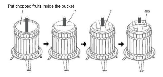
7. Place the nylon washer (3) on top of the Pressure Plate Assembly, as shown in the illustration. Screw on the trunnion (2), push the handle into the trunnion, and
