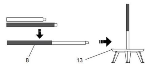
4. The base of the press should be screwed to a firm, solid floor or base, using the holes in the feet. (screw not included)
