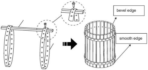
2. Wooden Pressing Plate (5) and Metal Pressing Plate (4) assembly with Screws (11).
