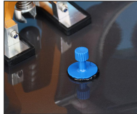
3. Attach the puller tabs to the depression, wait about 2 minutes
