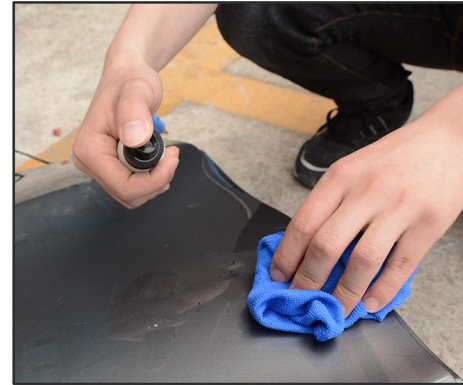
1. Clean the surface of the depression
