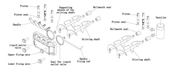
Note: Daub vaseline at the corresponding places when installing the pistons, piston seals, stirring shaft and bellmouth seals, for often using vaseline can prolong the service life of the components.
