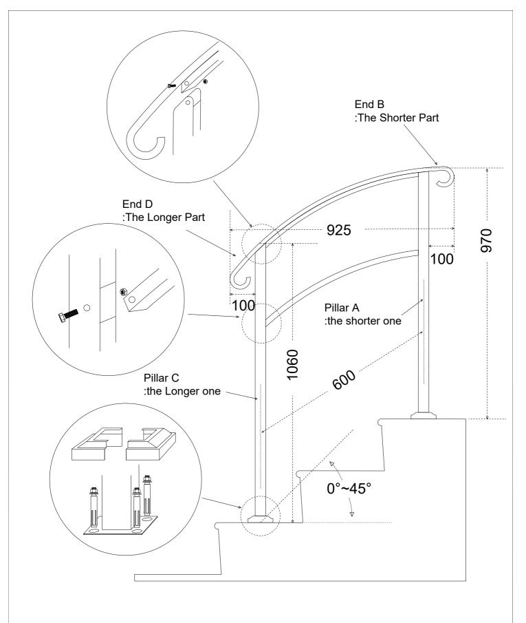
Pillar A should be attacked under End B (Uppper Stair)
