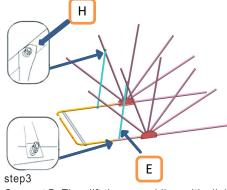
Connect D. Then lift the assemblies with all ribs and connect Cacross the Aor B frames
