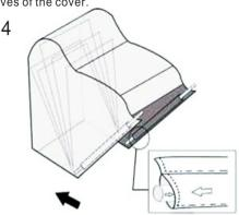
Let the last C tube pass through the ground sieeve of the cover and connect it with assembly A and B
