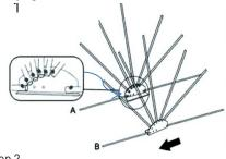
Step 2 Connect the E tubes on to the A&B parte with angled ends on upper rib using F,G & H fasteners.
