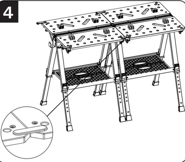
If desired, multiple units can be locked together side by side or end to end with the enclosed joiners.
