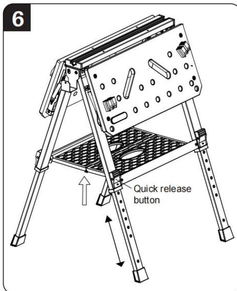
According to the arrow on the picture, it is convenient to quickly fold and shrink the leg
