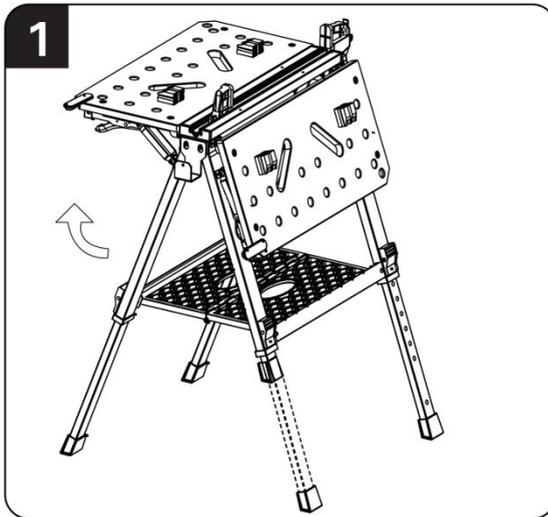
**NOTE:** Before using, check that the table is horizontal. To use as a work bench, press leg button to extend the legs to the top position, fully open the legs and pull the table top upward to make a work surface.
