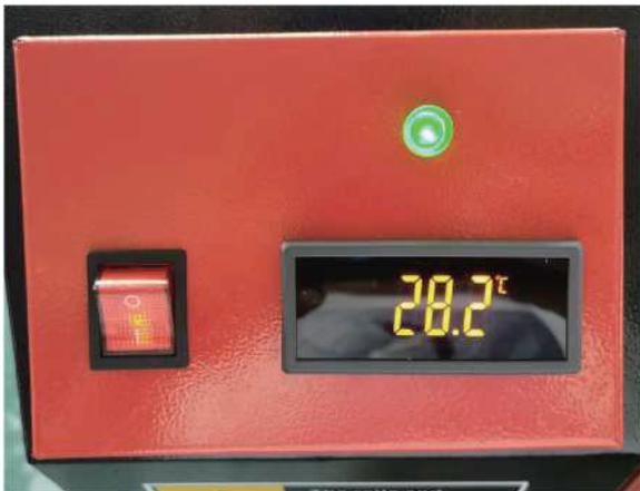
★ Please note that the water temperature should not exceed 35 degrees Celsius during use, otherwise the laser may be damaged. When the ambient temperature is about to drop below 0 degrees Celsius, please replace it with antifreeze liquid to avoid damage to the carbon dioxide glass laser.
