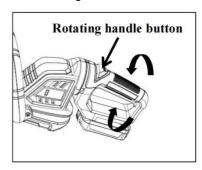
**Note:** The trimmer will only operate at one of these locked positions. The handle is locked when the rotating handle button is securely in place and the handle will no longer move to either side.
