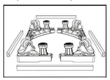
4. Insert stainless steel square tube and adjust to the proper size, then lock 4 buckles.
