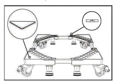
6. Rotate to the proper height to keep the base flat.
