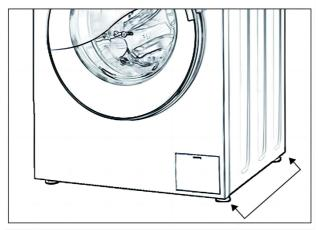
3. Adjust the length of the dollies according to the measured furniture width and tighten the hand screw nut.
