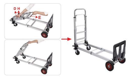
5. Hold the F lever pull it inward, while holding the handle G with your another hand, pull the frame up and out.
