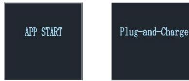
Press and hold on the charging panel again, and the display screen will display Plug and Charge to enter the Plug and Play charging mode. Open the Location, Bluetooth, and Wifi of the mobile phone. If the charging device is in standby state, the APP will automatically search for the charging device and the device name will be displayed.
