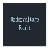
Note: When the voltage is detected to be below 175V, the charging current will be reduced by half.
