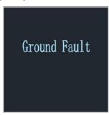
4.2 **Ground Fault:** The ground wire is not connected or the ground wire is poor. When this alarm message appears, please check if the grounding is normal. After ensuring reliable grounding, press the H button for 5 seconds to resolve this fault.
