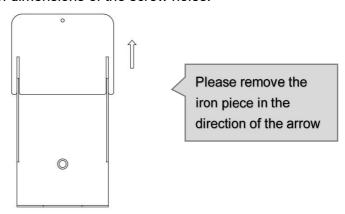
b.Select the installation location of the device. The lowest position of the equipment is a wall mounted fastener 1200 mm above the ground. Dimension unit is mm.
