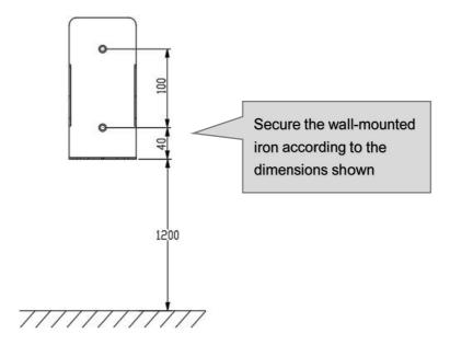
c.Drill 2 holes with a diameter of 8mm according to the location of the fixed screw holes of Wall mounted fasteners, and tap in the expansion rubber plugs. Fix the mounting plate with nuts to fix the chassis.
