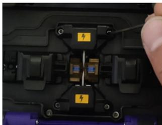
(3) Install the new electrode into the electrode slot, fit the electrode cover and slowly tighten the screws.
