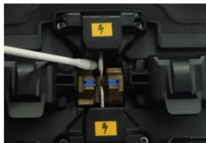
(1) Turn off the power of the fusion splicer and open the windproof cover.
