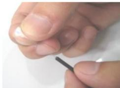
After stripping the fiber, a dust-free paper moistened with high purity alcohol is used to remove debris from the coating layer, starting at the interface between the coating and the bare fibre and rotating in a circular direction towards the bare fibre.
