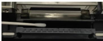
Dust and dirt are easy to deposit on the heater, please clean the heating plate regularly with a dry cotton swab.
