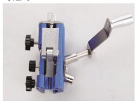
8. Pull carbide out and put chain forward to sharpen the next tooth, The thumb screw should not be adjusted again, This insures all teeth are sharpened the same amount making the entire chain uniform and precise.
