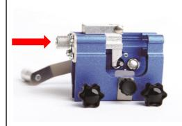
3. The carbide should now be inserted into the guide. The tool should rock on the carbide Find balance point where neither end of tool touches chain. Tighten the side screw to holdthe pawl against the sawtooth.
