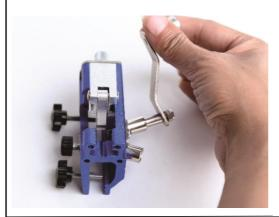
7. Pull carbide out and tighten rear thumb screw approx.
