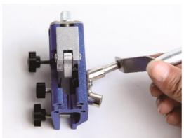
4. Rotate the handle to get the tooth sharper. Pull out carbide. Pull chain forward to test that it moves freely through tool.If nit, repeat step 3 and find correct balance point.
