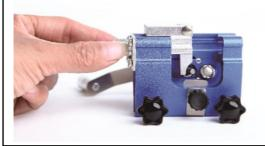
6. Tighten the Rear thumb screw until the Pawl pushes against the chain's tooth.
