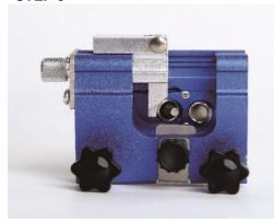
5. Reinsert earbide into guide and chain tooth. Tighten middle side set screw to apply sight side pressure via the spring elip to keep the chain vertical if needed.
