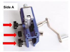
1. Place chainsaw on flat surface pointing towards you. Place tool on saw with side set screws on side A. Make sure 3 black screws are loosened.
