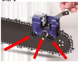
2. Put the sharpener on the saw blade and tighten 3 black screws. Insert the burr to the sleeve guide, stucking with the sawtooth.
