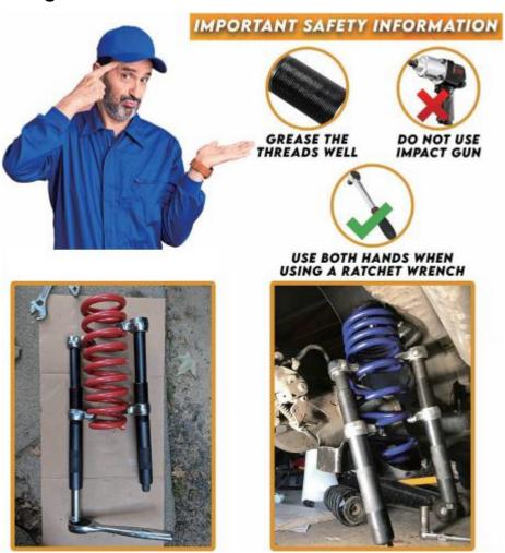
1. Fix the shock absorber assembly on the special tool, tighten the compression nut, and pay attention to the spring status at all times.
