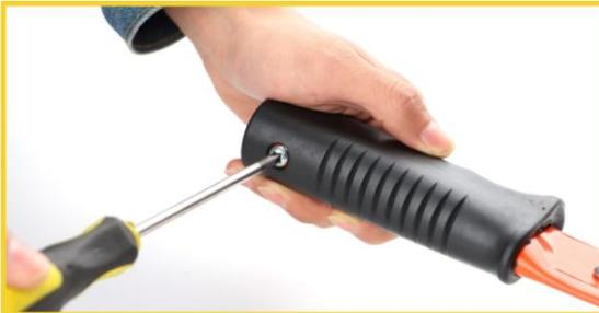
1. Remove the fixing screws from the black handle of the saw with hooks and set them aside for later use.
