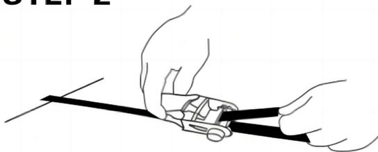
Pull webbing through, removing the slack.
