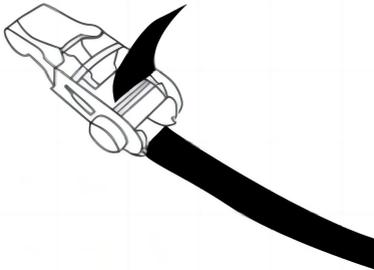
From bottom, thread webbing though slot in center spool of closed ratchet.
