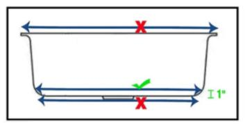
2.Confirm The Length and Width of The Sink Please note that the measured length and width of the sink should be 0.3 inches larger than the Sink Grid.
