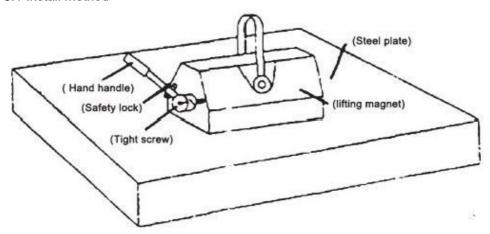
In the first step, place the permanent magnetic lifter in the center of the steel.
