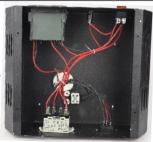
2.Check the resistance of the heating coil like this:If 110V,the resistance is about 8?. If 220V,the resitance is about 30?.I1 the resistance is infinite,that means the heating coill is broken,then you need to change a heating coil.
