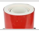
4. Take off the broken heating coil and winding a new heating coil on the furnace chamber. Don't forget the insulating rod! This is the finished furnace chamber with heating co"
