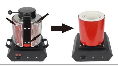
3. After take out the flange, you can take out the furnace chamber, here is the furnace without furnace chamber.
