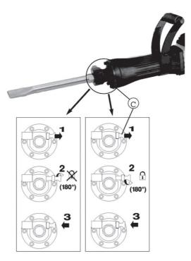
The chisel is locked by the chisel lock(C). To insert and remove the chisel, please follow the steps below:
