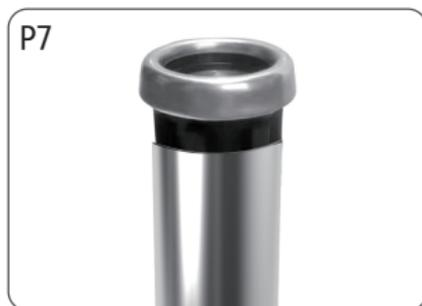
Press the mounting sleeve into the round tube
