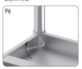
Twist the shelf bolts Torque is greater than or equal to 25 N•m
