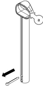
9. Remove the MOUNTING TUBE from the Hose Reel and slot it over the WALL BRACKET. Align the holes in the HOUSING with the holes in the WALL BRACKET
