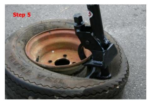
5. Continue to turn clockwise until bead is broken loose from rim. If necessary, Repeat this process in 2 to 3 locations on each side of the wheel until entire bead is broken.
