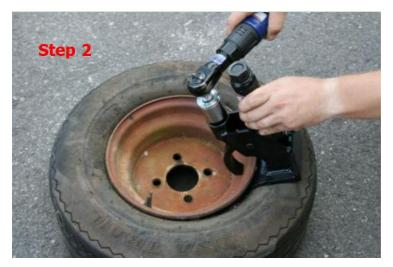
2. Tighten rim clamp jaw until "snug" with hand wrench. Make sure bead breaker teeth and foot are against bead.
