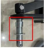
5.Install the wheel set(C), insert the pin(M) and bend it.
