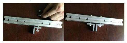
3.Attach dog (No.3) to hinge plates (No.4) with bolt, washers and nut (No.9,12 and 8). Tighten all bolts.
