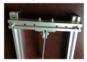
5.Install leveling screws (No.6) into cross bar (No.2) slotted end of screw is in the same direction as the head of the carriage bolts.
