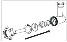
2. Attach the grinder head to the motor housing.
