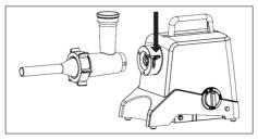
3. Press down the locking handle to make sure that the grinder head is locked firmly.
