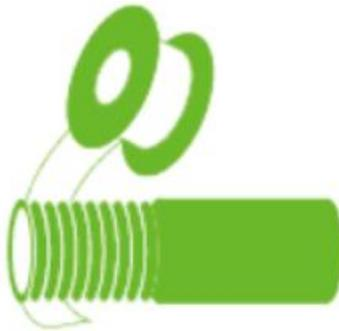
**Note:** If you install and remove the connector yourself and the switch is not vertical, try increasing the number of winding laps of waterproof tape.
