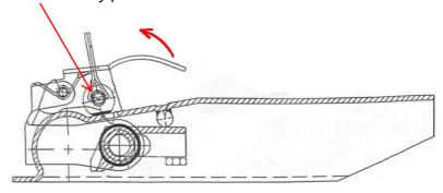
To open, pull the coupler handle and rotate. Place coupler on ball. When ball is completely nested in ball socket. Release the coupler handle until handle is in locked position. Plug in the safety latch.
