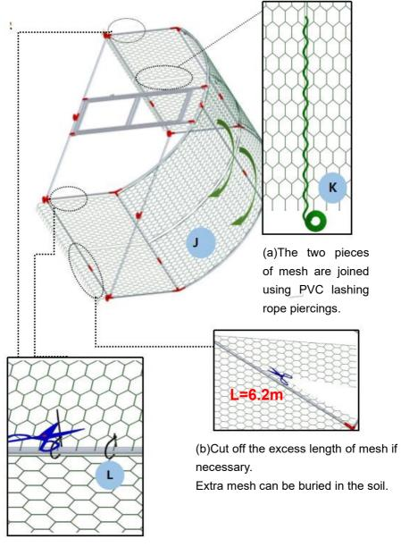
(c)Secure the mesh to the frame with cable ties.
