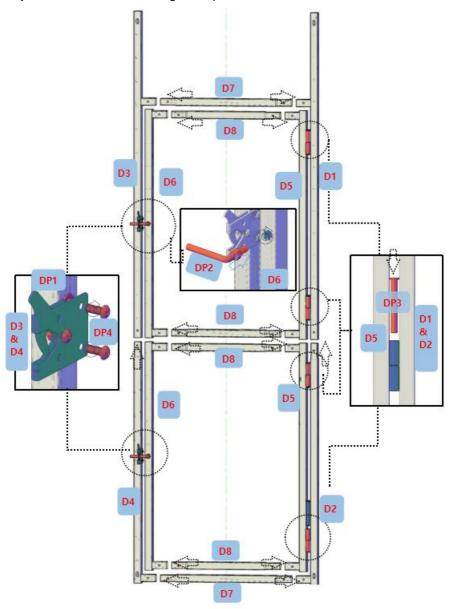
**Step7:** Attach the door to the frame.
