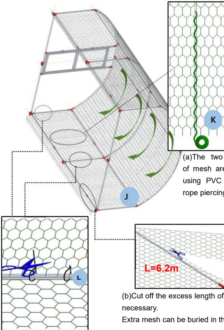
(a) The two pieces of mesh are joined using PVC lashing rope piercings.
