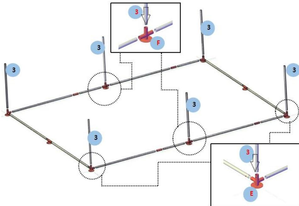
**Step4:** Install the beam according to the part number in the picture below.
