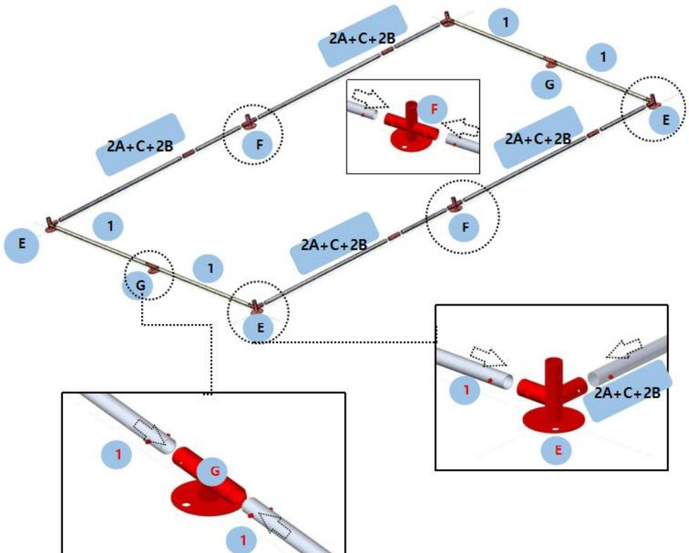
**Step3:** Install the column according to the part number below.
