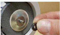
Inspect the new stone for cracks and damage to either the front face or the edges before fitting.
