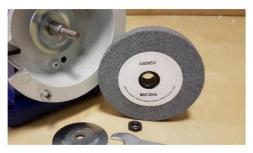
Remove the plate flange and carefully remove the stone.
