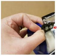
Attach the two Eye Guards using the small screws, washers and locking washers.
