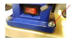
Secure the Grinder to a bench. Either screw through the four holes in the base.
