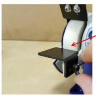
Attach the two work tables using the wingnuts and washers.
