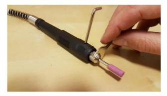
To fit a tool into the flexible shaft:
