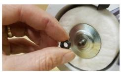
Carefully slide the mop onto the shaft, replace the plate flange, the nut and tighten against the rotation of the mop.
