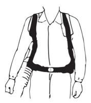
Position the hip strap at hip level, not too far down the stomach. Tighten the hip strap so you can feel the weight of the appliance resting on your hips.
