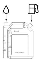
■ Tilt the mixing container ② to the side so that the filled oil can flow into the chamber with the petrol.
