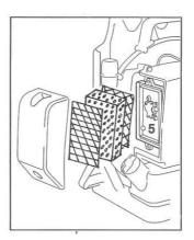
Dirty air filers reduce engine power increase fuel consumption and make starting more difficult.
